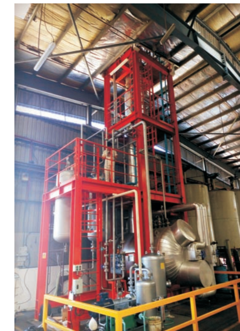
Skid-Mount MEG Recovery Plant used Winpak-1 structured packing constructed in Malaysia by PCC.
